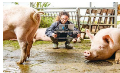
Prototype of a multi-spectrum camera enables FiBL livestock researcher to detect even the smallest injuries in pigs. Photo: Marion Nitsch
