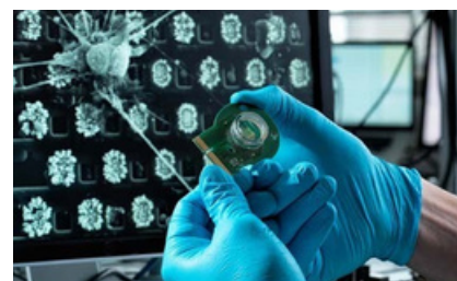
High-density array of thousands of micro-electrodes, which are used for electrophysiological recordings at sub-cellular resolution. Photo: Pino Covino for ETH Zurich, image on the monitor: Branka Roscic, Douglas Bakkum / ETH Zurich.
