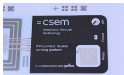
Roll-to-roll printing technologies applied to mass manufacture a battery-free and flexible sensing platform.
